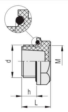
$\begin{array}{lll} d & = M \ 42x2 \\ D & = 53.5 \\ h & = 15 \\ L & = 26 \\ M & = 38 \\ s & = 46 \\ Weight (g) = 21 \end{array}$
